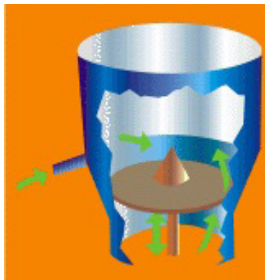
Fig.9: Rotating Disk Granulator
